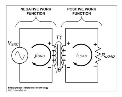
**ABSTRACT:** A typical Alternating Current (AC) transformer utilizes a principle of transferring electrical energy called *mutual electromagnetic induction*. This effect described as Faraday's Law of Induction (1831) permits a near equal amount of REAL power to be transferred between the input coil and the output coil. The "near equal amount" is the result of imperfections or losses in the transformer causing the efficiency of the same transformer to approach, but never exceed 100%.
