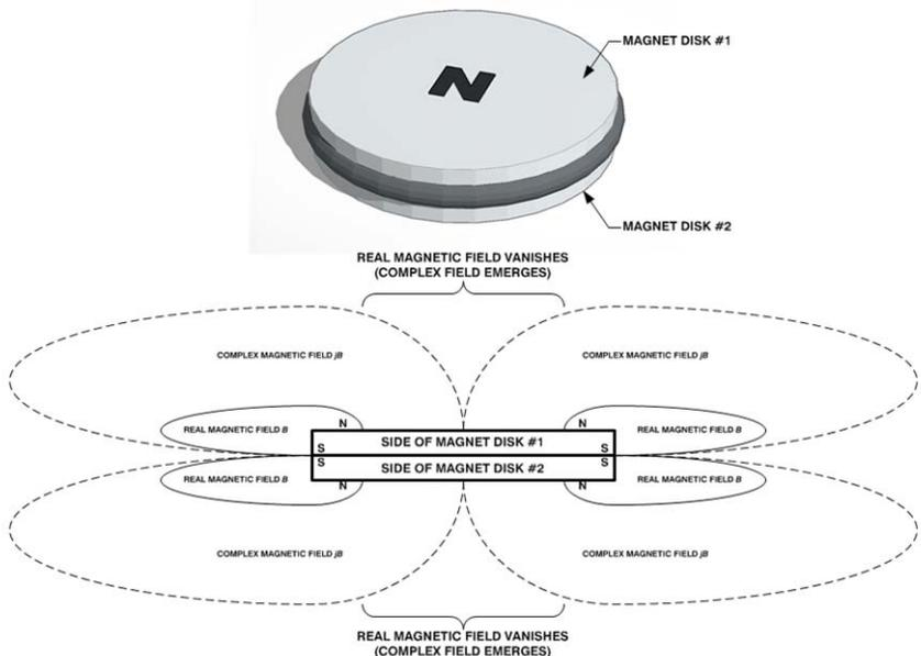
**REAL & COMPLEX MAGNETIC FIELDS PRODUCED BY DISK MAGNETS**
